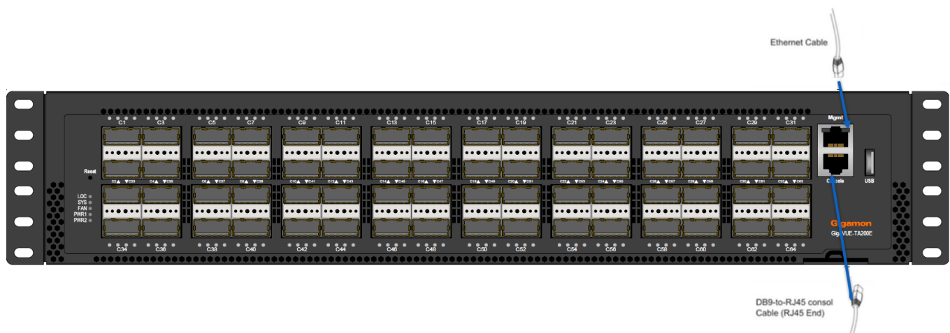
Figure 5 Connecting the Console and Management Ports
